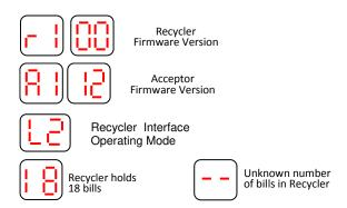
By default, in normal operation, the display always shows the number of bills currently held in the Recycler available for use as change. If the recycler has lost count of the number of bills for whatever reason, then a double dash will be displayed. The recycler will recalculate and display the number momentarily. This could take up to 1.5 minutes.
